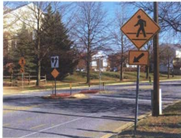
DPW&T Standard 700.05 (above left) and an existing pedestrian refuge along Riedel Road in Anne Arundel County (above right). A pedestrian refuge can often be the single most important enhancement for improving the safety of a pedestrian crossing when multi-lane roads are involved.
