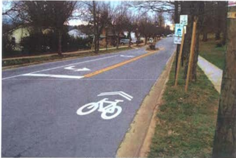
Shared lane marking
